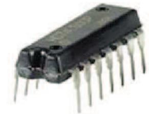
Pin spacing is 0.1" x 0.3"; chip is about 15mm long
