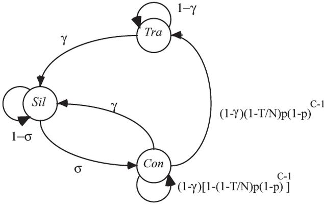
Figure 2. PRMA terminal state transition diagram.
