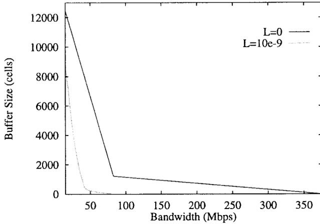
Fig. 9. Buffer/bandwidth tradeoff for two classes.
