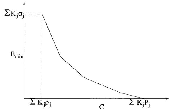
Fig. 3. Optimal buffer/bandwidth tradeoff curve.
