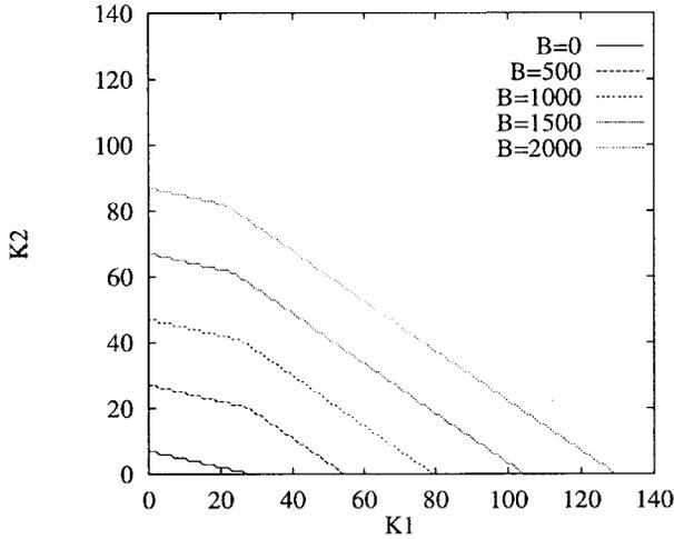
Fig. 11. Admissible region for two heterogeneous classes:  $T_{on1} \approx T_{on2}$ .
