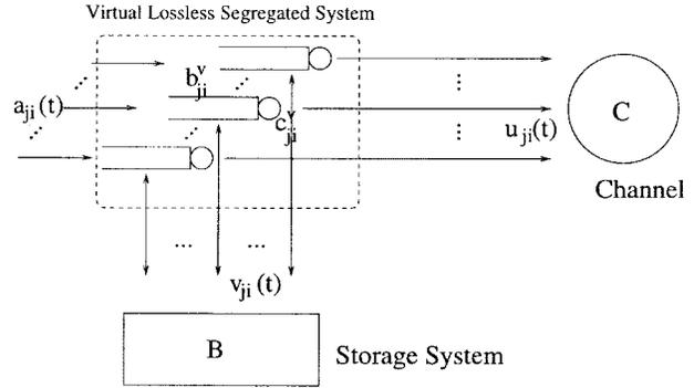
Fig. 7. Buffer/bandwidth separation via virtual lossless segregated system.
