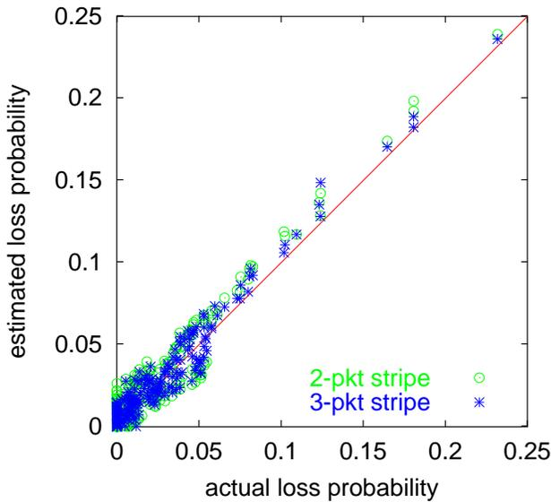
Fig. 5. Inferred vs. actual link loss rates in simulations. 3 packet and 2 packet substripes. Scatter plot for 100 experiments.
