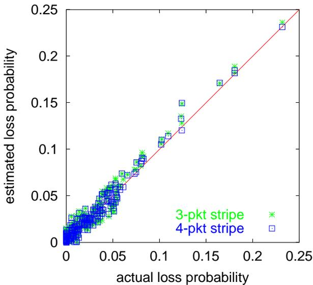
Fig. 6. Inferred vs. actual link loss rates in simulations. 4 packet stripes and 3 packet substripes. Scatter plot for 100 experiments.
